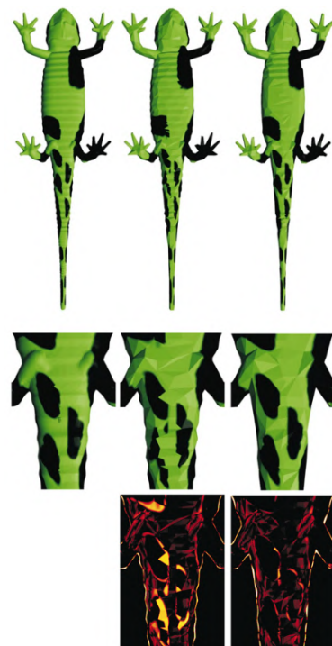
Figure 4.2: Comparison of the original textured mesh (left), geometry-based (middle), and image-based simplification (right) with displacement heatmaps. Image credit: Lindstrom et al. [49].
