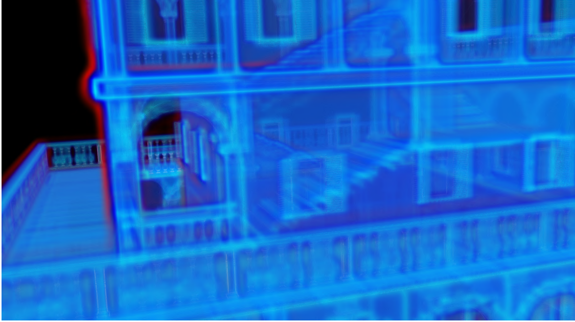
Figure 4.3: The distance field to a free palace mesh [75] with 1M triangles and 500K vertices on a grid \bar{G} with resolution 600^3 completed in about 21 seconds on AMD Ryzen 7. The exported voxel .vti file (ASCII) has 1.1 GB.
